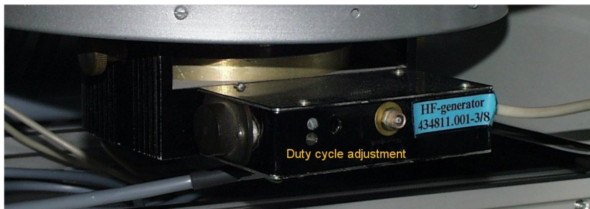
Figure 12: HF oscillator adjustment (Dissociator in the rack)
